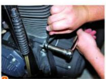
If you have forward controls, chances are your shift linkage is long enough for this kit. If you are running mid-controls, Widow Maker Industries supplies a new linkage. Either way, the linkage needs to be removed from the shift lever.
