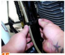
...and down the left side down tube. Note that I used the stock cable clamps to secure the cable.
