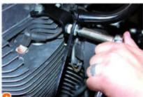
Now it was time to mount the actual shift arm. This photo is an excellent reference showing how the thicker plastic washer went on first, followed by the shifter arm, then the thinner plastic washer. Finally a metal washer and a lock nut were placed on and tightened down.
