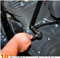
The shift linkage was then installed onto the bottom of the shift arm. The heim joint on the linkage was attached to the shift arm after test fitting for the correct and moreover, comfortable length.
