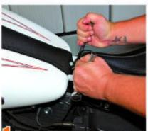
The first step was to remove the seat and lift the tank. On this setup, the bike has H-D's spring seat which permits only removing the rear tank and the front seat mount bolt.
