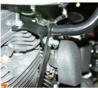
Once the first lock nut was torqued down, the second lock nut was installed. This adds extra security and the photo shows how it looks once it was installed.
