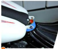
From here, I used a roll of painter's ta to prop the tank up. This is easier on the tank and it provides enough clearance to get to the engine mount bolts.
