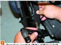
From here, I pulled off the shift lever bolt and slid the shift lever off and then removed the shift mechanism.
