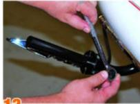
The factory shift lever mount and perch were then installed onto the shift arm. I found it easiest to thread the screws just a bit to close both sides and then slid it down the arm. This gave me the ability to adjust it while I was tightening it so that I could get it in the right position.
