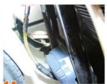
Now I was ready to route the clutch cable. The kit is designed to use the factory cable by just rerouting the cable. This photo illustrates how I routed the cable up the right side down tube...
