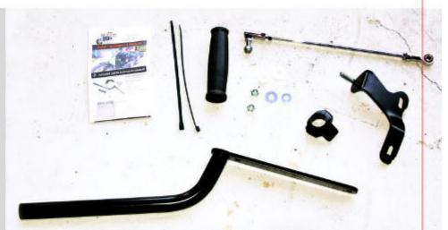
As you can see, this is a full kit; meaning that everything is included for your install. The main pieces are the shift mount, the shifter assembly, the shift linkage, new mirror mount, and a rubber grip.
